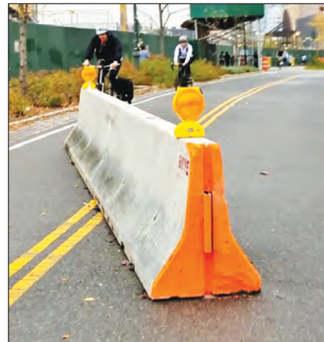
Photo from Traffic Safety Warehouse An example of Jersey barriers used to deter vehicles is shown.
